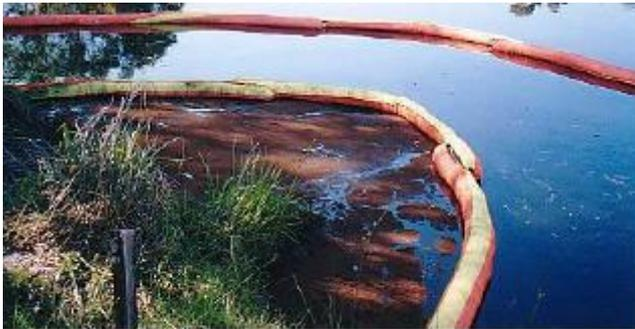
*Booms contain spill, Absorbent Peat encapsulates spill*
